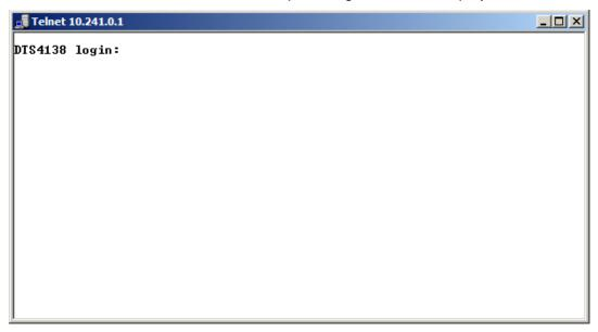
To start the menu, dts must be logged in as user. The standard password is dts. (Changing the password  $\Rightarrow$  see chapter "6.5.20 General settings").
