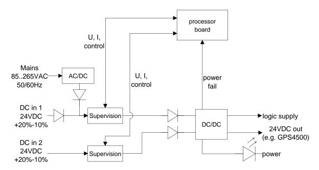
The mains supply and the DC in 1 input are internally linked, but protected against "Back powering".
